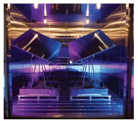
Mirrors undergoing lifetime testing in the environmental chamber
