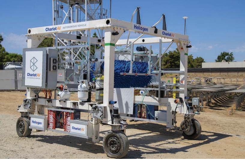
Autonomous cleaning vehicle, Chariot AV, at our testing and demonstration facility in Lancaster, California
