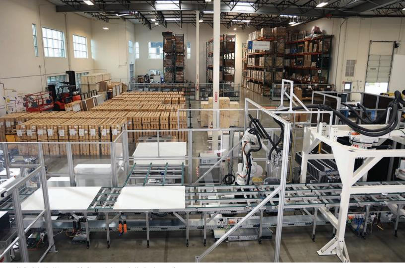
Heliostat robotic assembly line and storage in the background
