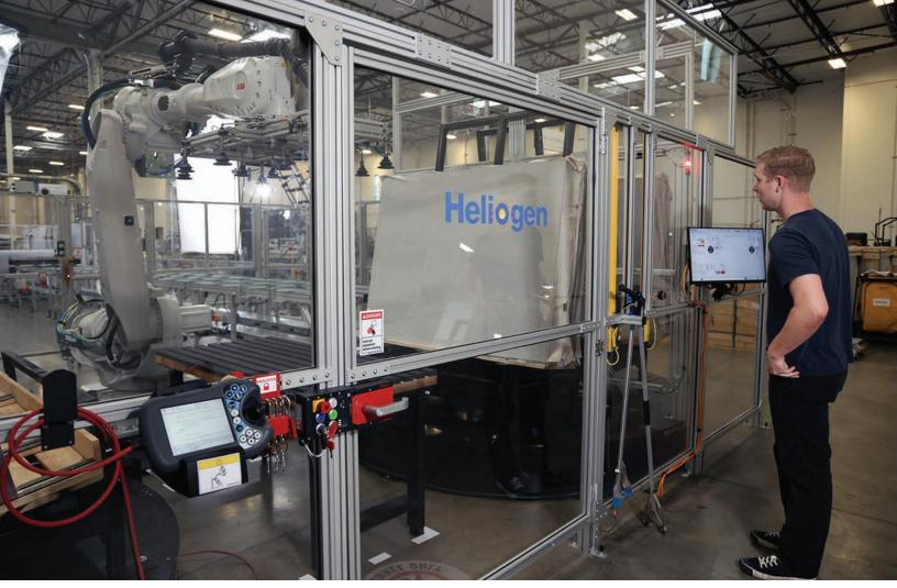
Operator inspecting heliostat assembly process
