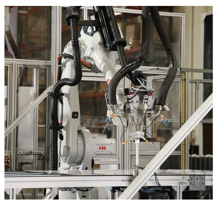
Robotic arm dispensing adhesive during mirror assembly
