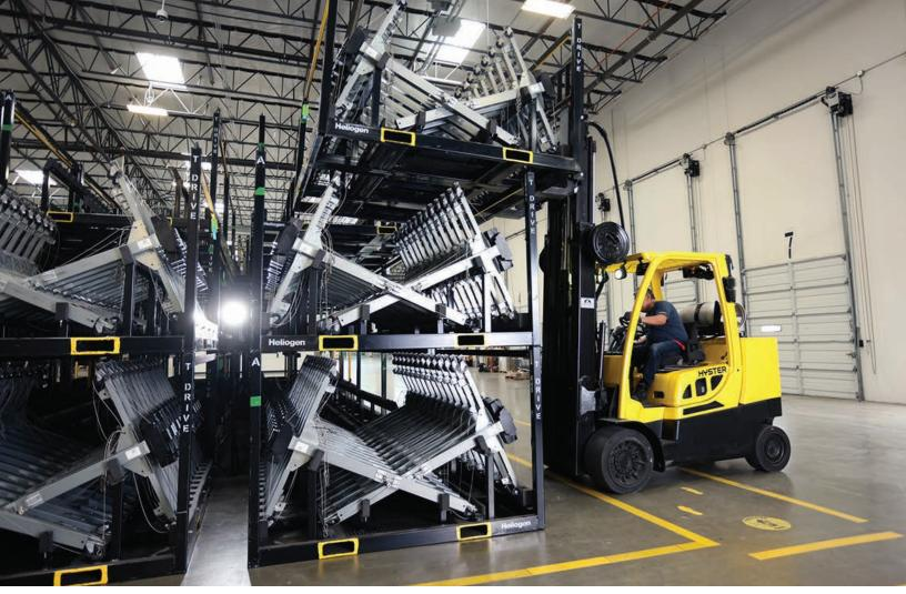
Finalized heliostat T-drives placed in reusable shipping containers
