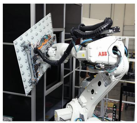
Robotic arm moving mirror to optical scanning system
